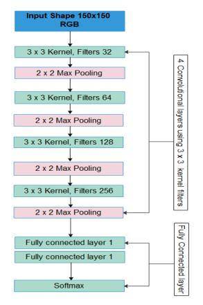
Fig. 4. Convolutional network architecture for fire detection
