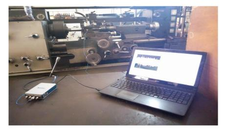
Fig. 1. Acquisition device
