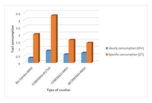
Fig. 14. Fuel consumption of crusher
