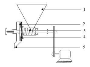
Fig. 10. Design of almond mill with carborundum stone
