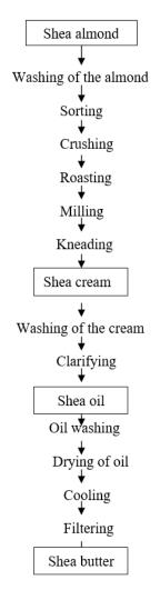
Fig. 13. Flow diagram of production of shea butter
