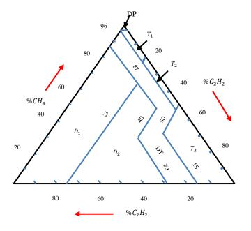
Legend:PD = Partial dischargeT1 thermal fault less than 300°CT2 = thermal fault between 300°C and 700°CT3 = thermal fault greater than 700°CD1 = low energy discharge (sparking)D2 = high energy discharge (Arc)DT = mix of thermal and electrical faults
