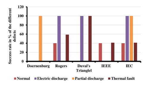
Fig. 2. Defect success rates using conventional methods
