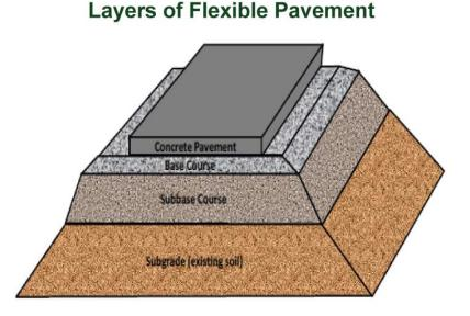
Fig. 5. Typical cross-section of a pavement structure and terminology of the different layers
