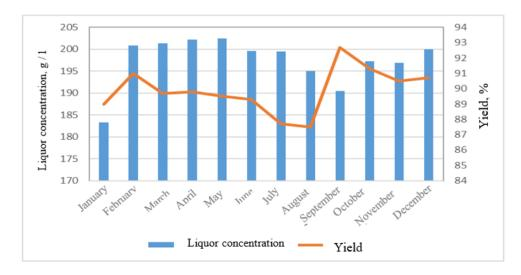
Fig. 10. Changes in alumina yield as a function of etching liquor concentration
