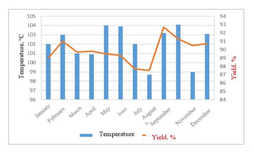
Fig. 8. Changes in alumina yield as a function of etching temperature
