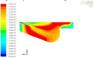
Figure 6: Temperature contour at 30 degrees below TDC
