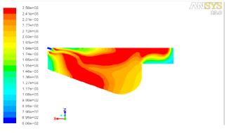
*Figure 5: Temperature contour at 27.5 degrees below TDC*
