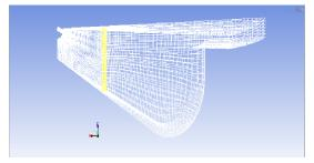
Figure 2: Mesh for the combustion chamber
