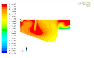
Figure 4: Temperature contour at 20 degrees below TDC.
