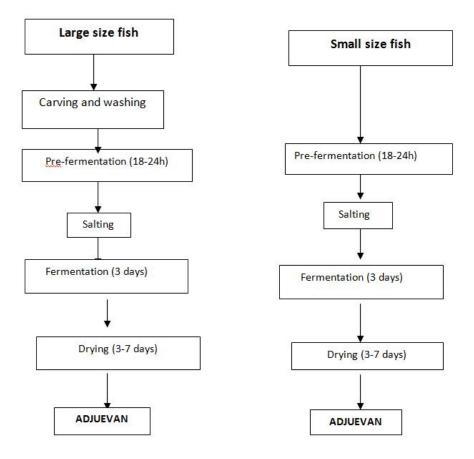
Figure 1: Adjuevan processing of large size and small size fish
