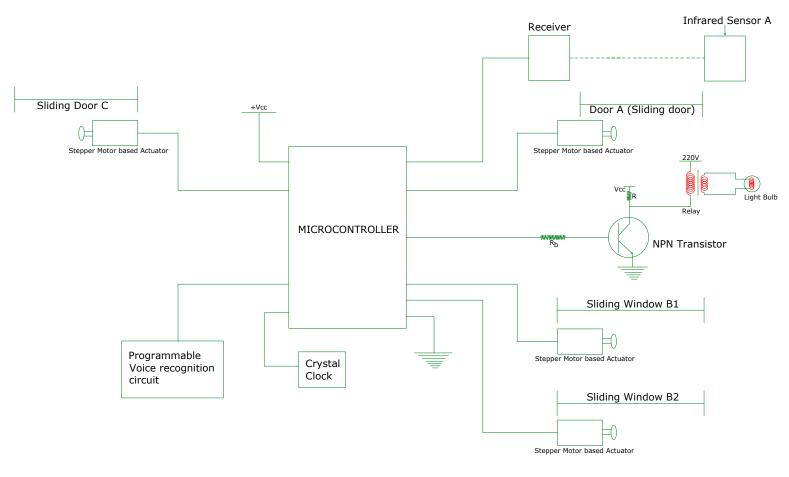
Fig. 6. A Microcontroller base BAS design
