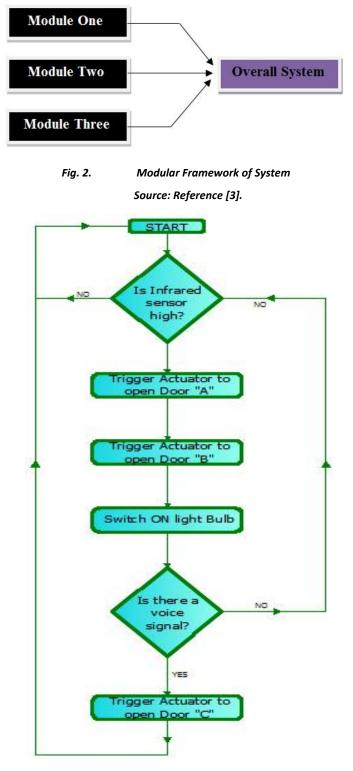
Fig. 3. Flow diagram showing the operation of the microcontroller
