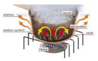
Fig. 2. The Mode of Heat Conduction
