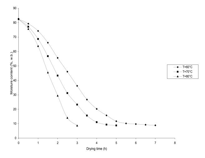
Fig. 1. Effect of drying temperature on the drying time and moisture content of mango slices.
