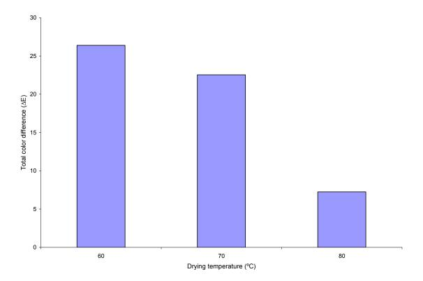
Fig. 3. Effect of drying temperature on total color change ( $\Delta E$ )
