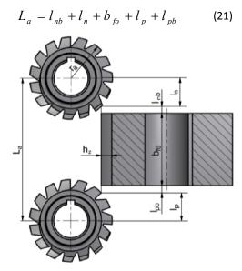
Fig. 7. Slope and run-out of the gear hob
