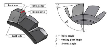
Fig. 6. Description of the hob gearing
