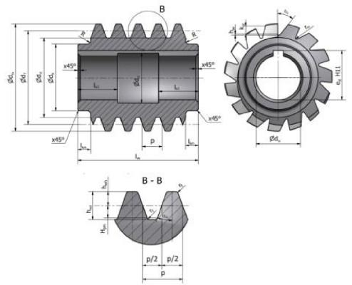
Fig. 5. Description of the gear hob structural elements
