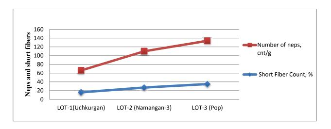
Fig. 2. Analysis of the number of neps and short fibers on the card sliver
