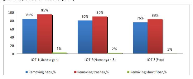
Fig. 1. Removal efficiency of neps, trash and short fiber in carding tape
