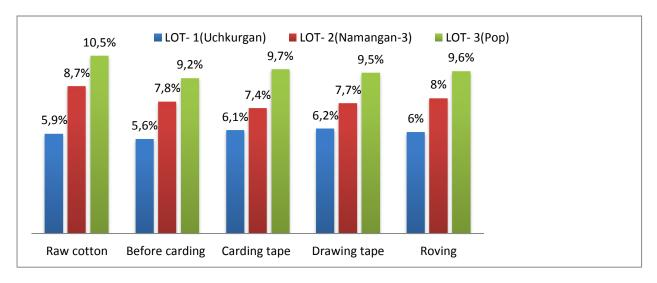
Fig. 3. Analysis of the amount of short fiber content (SFC) in the spinning process at the transitions, %
