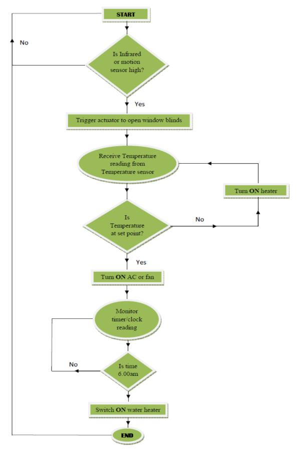
Fig. 4. Flow diagram showing the operation of the microcontroller
