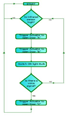
Fig. 3. Flow diagram showing the operation of the microcontroller
