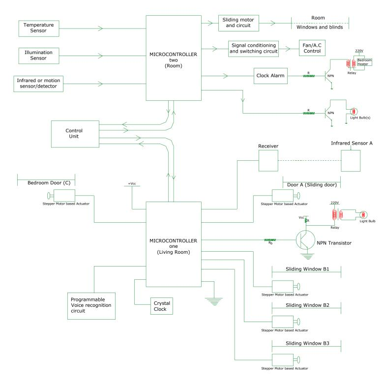
Fig. 7. A Microcontroller base BAS design
