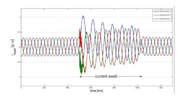
Fig. 10. Three-phase load current swell waveform without DPFC
