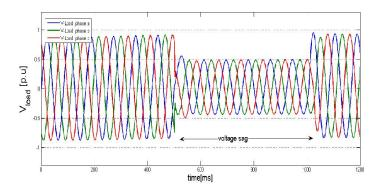
Fig. 8. Three-phase load voltage sag waveform
