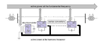
Fig. 2.Active power exchange between DPFC converters
