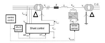
Fig. 3. DPFC control structure
