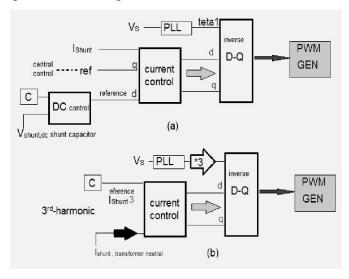
Fig. 6. The shunt control configuration: (a) for fundamental frequency (b) for third-harmonic frequency
