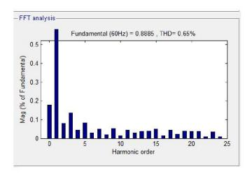
Fig. 13. Total harmonic distortion of load voltage with DPFC
