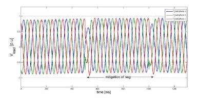
Fig. 9. Mitigation of three-phase load voltage sag with DPFC
