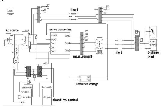
Fig. 7. Simulation model of the DPFC
