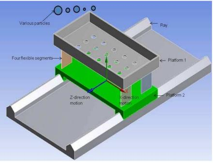
Fig. 2. A system diagram of a novel compliant vibrating mechanism
