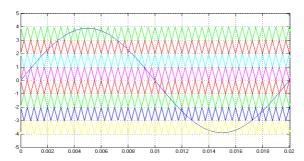
Fig. 4. Carrier arrangement for Alternate Phase Opposition Disposition PWM strategy
