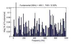
Fig. 16. FFT plot of 9-level Hybrid H Bridge MLI Using PSPWM Strategy
