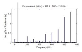
Fig. 10. FFT plot of 9-level Output Voltage waveformHybrid H Bridge MLI Using PDPWM Strategy
