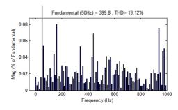
Fig. 14. FFT plot of Hybrid H Bridge MLI Using PODPWM Strategy
