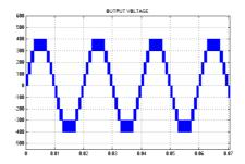
Fig. 15. Simulated 9-level Output Voltage waveform of Hybrid H Bridge MLI Using PSPWM Strategy
