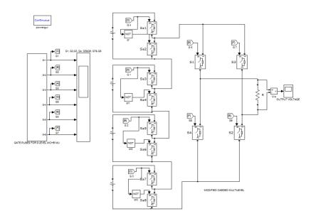
Fig. 6. Simulink Modeling of the Hybrid H-Bridge Multilevel Inverter
