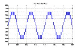
Fig .11. Simulated 9-level Output Voltage waveform of Hybrid H Bridge MLI Using PODPWM Strategy
