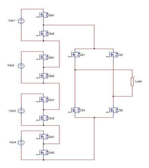
Fig. 1. 9-Level Hybrid H-Bridge Multilevel Inverter
