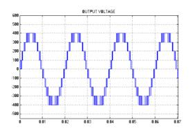
Fig. 9. Simulated 9-level Output Voltage waveform of Hybrid H Bridge MLI Using PDPWM Strategy
