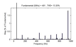
Fig. 12. FFT plot of Hybrid H Bridge MLI Using PODPWM Strategy
