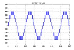
Fig .13. Simulated 9-level Output Voltage waveform of Hybrid H Bridge MLI Using APODPWM Strategy
