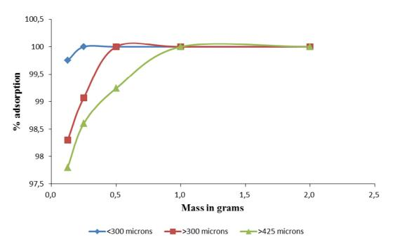
Figure 2: Effect of biomass dosage and particle size on adsorption of Cu (II) ions
