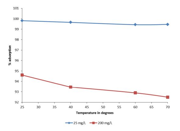
Figure 5: Effect of temperature on % adsorption of Zn (II) ions by 0.5 g of E. crassipes
