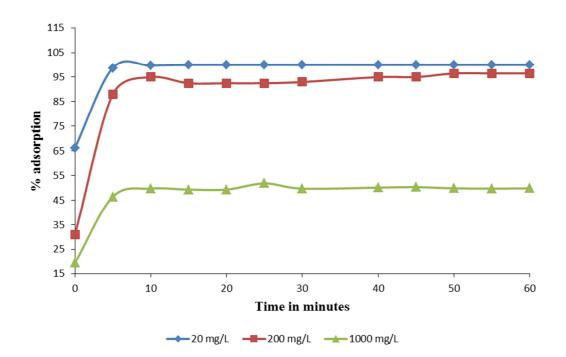
Figure 4: Effect of concentration and contact time on adsorption of Zn (II) ions by 0.5 g of E. crassipes
