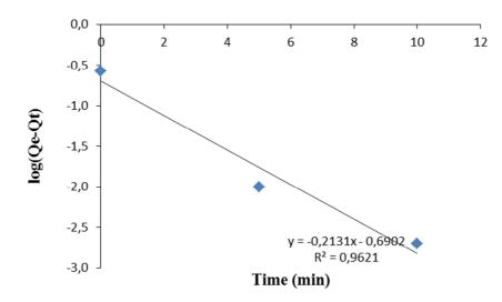
Figure 6(a): Pseudo-first-order plot for adsorption of 20 mg/L of Zn (II) onto E. crassipes
