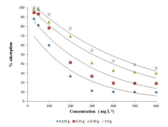
Figure 3: Effect of initial concentration of Zn (II) ions on adsorption by E. crassipes
