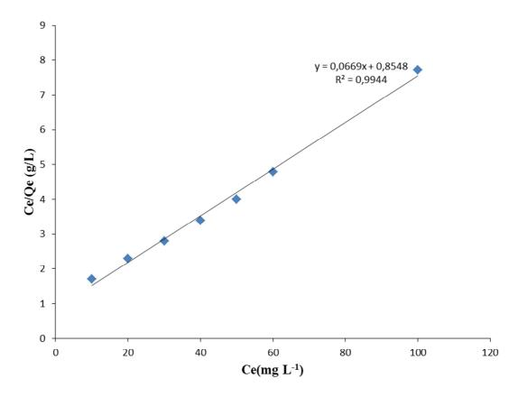
Figure 7(a): Linearized Langmuir isotherm for adsorption of Zn (II) ions by E.crasippes
