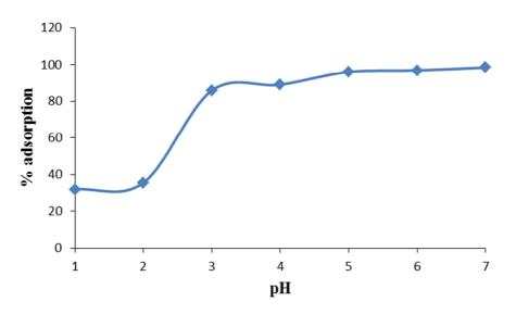
Figure 1 : Effect of pH on adsorption of Cu(II) ions onto E.crassippes
