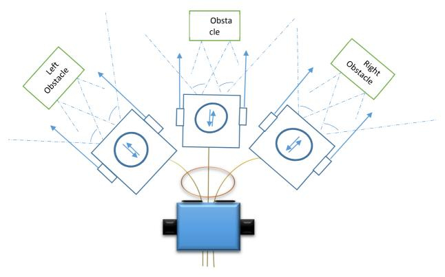
Fig 3.0 Robot Multi directional Search path
