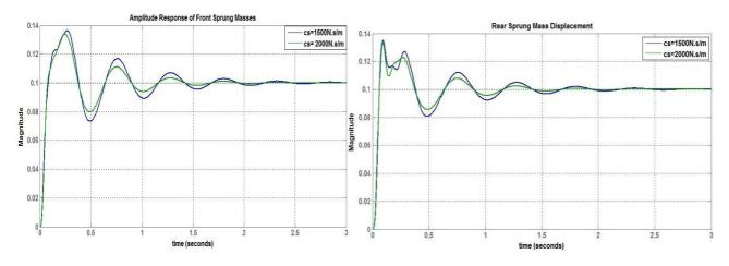
Fig. 7 Amplitude Response of Half Car Model Front Sprung MassFig.8. Amplitude Response of Half Car Model Rear Sprung Mass
