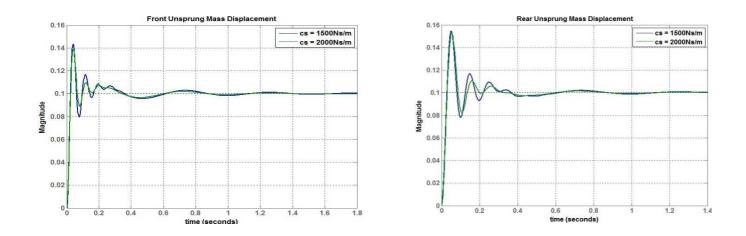
Fig. 11 Amplitude Response of Half Car Model Front unsprung Mass Fig. 12. Amplitude Response of Half Car Model Rear unsprung Mass
