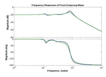
Fig.13. Frequency Response of Half Car Model Front unsprung Mass
