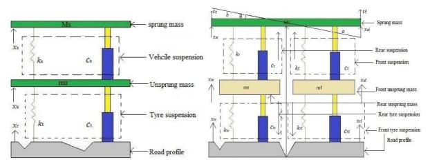
Fig. 1 Two Degree of freedom ModelFig. 2 Four Degree of freedom Model
