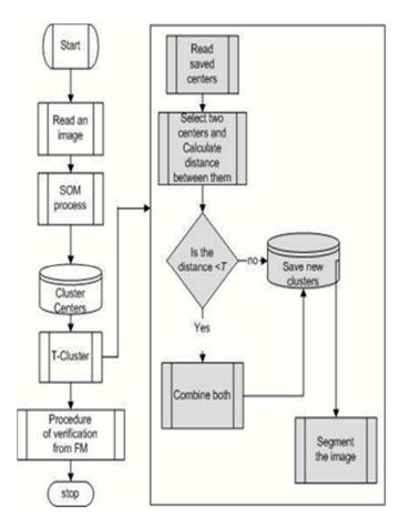
Fig 4: SOM and T cluster sequential process
