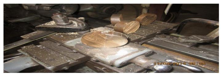
Fig 2. Cutting and Turning of the Metal Brass
