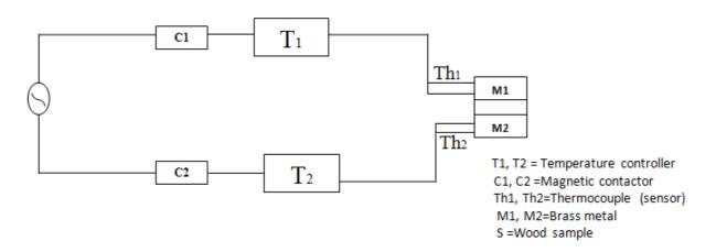
Fig 3 Block Diagram of the electrical set-up
