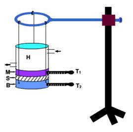
Fig 1 Lee's disc set-up Ref [23]
