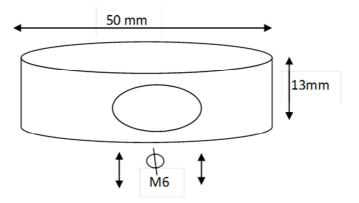
Fig 3. The metal disc with dimension
