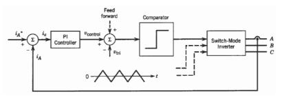
Fig:2 Fixed Frequency Control
