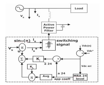
Fig: 7: Structure of wavelet Controller for APF
