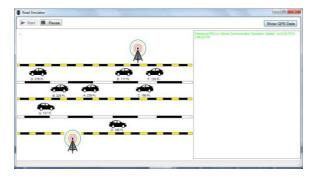
In a typical scenario of Vehicle to Roadside Unit Communication, Roadside Unit communicates with all the vehicles in the network. These vehicles have its own location information. This location information of vehicles is shared with Roadside Units in the region. When simulation starts, RSU communicates with the vehicles in the network. Next step would be to perform an accident of a vehicle, which can be done by clicking on a vehicle. When we click a particular vehicle a dialog box will appear
