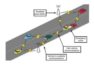
Fig. 1.1 Communication in VANET (V2V and V2I)
