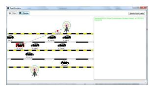
'B' met with an Accident which is shown in Red area. This B Vehicle then communicates with Road Side Unit (RSU). RSU will get all the location information through GPS. RSU then calculates the position of the vehicle by using great circle algorithm and bearing angle.
