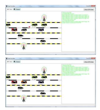
The simulation results shows the distance between the vehicle and bearing angle which met with an accident and the affected vehicle. Thus, giving the relative position of the vehicles as shown in the output screen. In the fig 7.6 we can see four different colored zones to show the status of the vehicles in the network. These four different colored zones are RED, ORANGE, and PURPLE, GREEN.
