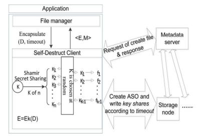
Fig 1. Uploading and Downloading file process
