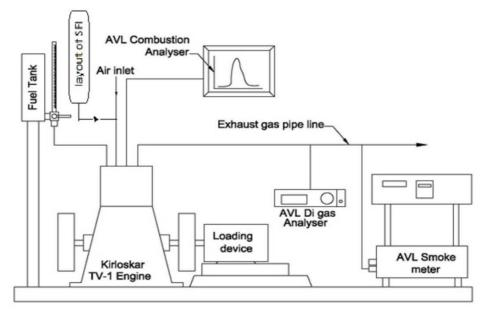
Figure 1: Layout of Experimental Setup with Secondary Fuel injection (SFC).
