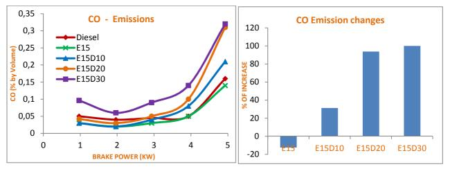
Fig 6: Brake power Vs CO Emissions.
