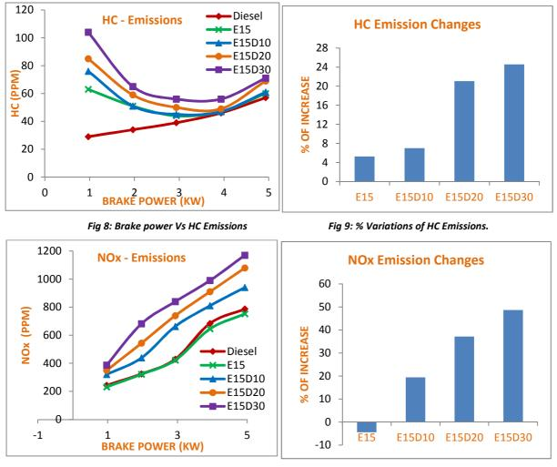
Fig 10: Brake power Vs NOx Emissions.
