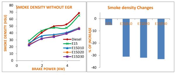
Fig 12: Brake power Vs Smoke Density.
