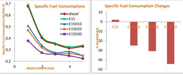
Fig 2: Brake power Vs SFC.
