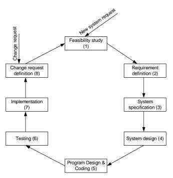
Fig. 1. Advanced Software Development Life Cycle system (SDLC)
