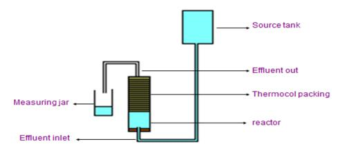
Fig. 1. Experimental Setup Of HUASB Reactor Design
