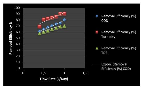
Fig. 2. Experimental Results for Efficiency of HUASB Reactor
