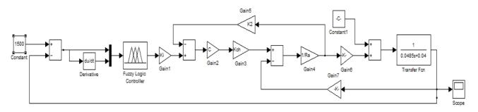
Figure 11. Simulink Model of FLC Control for Chopper fed DC Motor
