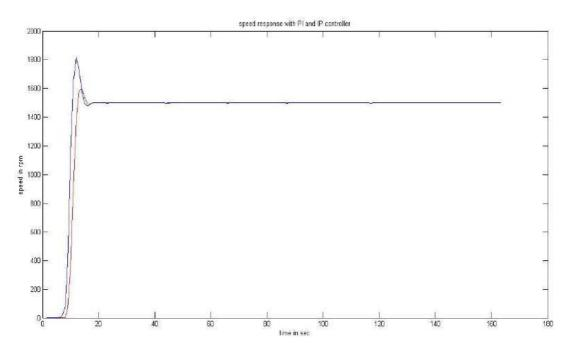
Figure 8. Comparison of Speed Response of Chopper fed DC Motor using P-I and I-P Controllers
