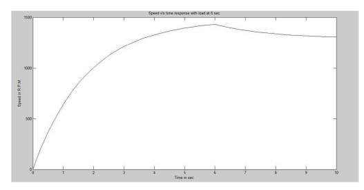
Figure 12. Speed Response of Chopper fed DC Motor using Fuzzy Logic Controller
