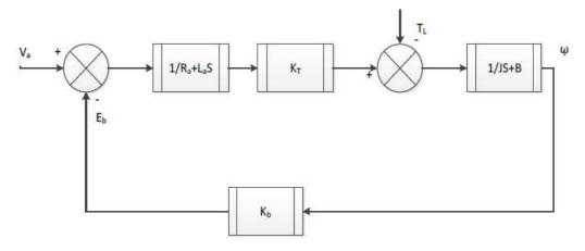
Figure 3. Block Model of Separately Excited DC Motor
