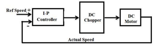
Figure 5. I-P Controller based Speed Control of Chopper fed DC Motor Comparative Analysis of Speed Response of Chopper Fed DC Motor using P-I and I-P Controller
