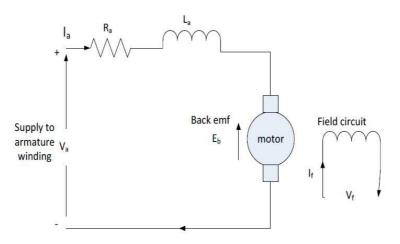
Figure 2. Separately Excited DC Motor Model
