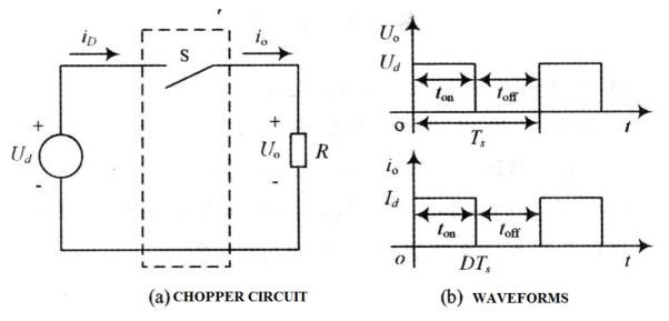
Figure 1. Chopper Circuit and its waveform
