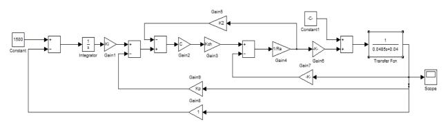
The MATLAB/SIMULINK Model for Speed Control of Chopper fed DC Motor using I-P Controller is shown below:
