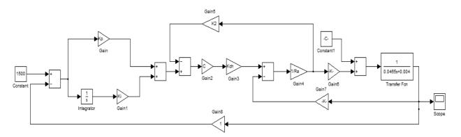
Figure 6. Simulink Model of P-I Control for Chopper fed DC Motor
