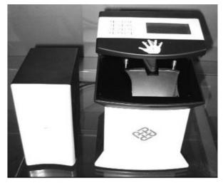
Fig. 2. CCD based palm print scanner
