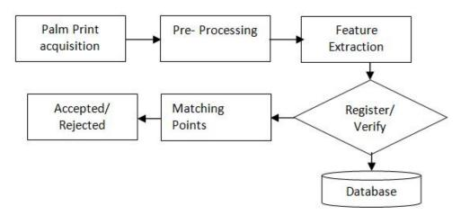
Fig. 1. Block Diagram of Palm Print Recognition
