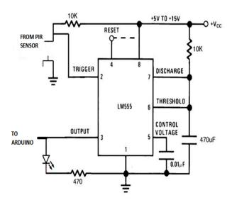
Fig. 2. Circuit Design for an LM555monostable mode
