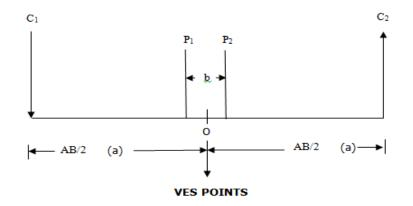
Fig 2: Schlumberger Electrode Configuration
