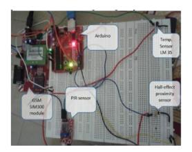
Fig. 3 Snapshot of the circuit
