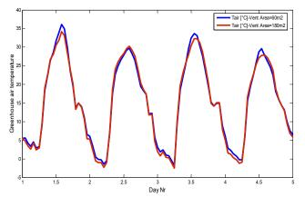
Fig. 3. The effect of ventilation area on greenhouse air temperature
