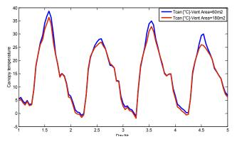
Fig. 4. The effect of ventilation area on canopy temperature
