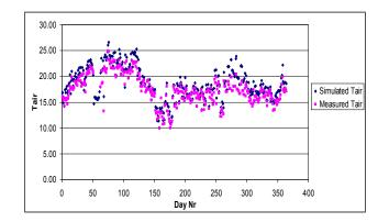
Fig. 2. Comparison of simulated and measured mean daily greenhouse temperature
