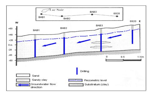
*Fig. 2. Hydrogeological section of the unconfined dune aquifer*
