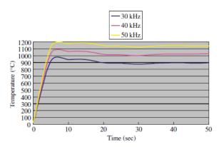
Fig. 1. Variation of surface temperature.[7]
