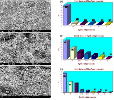
Fig. 9 SEM photographs of workpiece materials before drilling a 50% Alumina, b 60% Alumina and c 70% Alumina [23]
