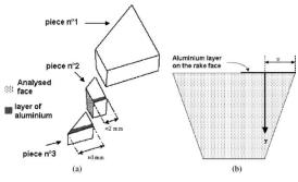
Fig. 6. Section of the carbide tool insert analysed. [30]
