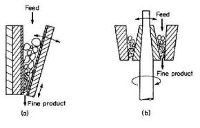
Fig.1.2.3 a) Jaw Crusher b) Gyratory crusher
