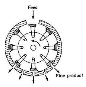
Figure 1.2.3 (c) Hammer mill
