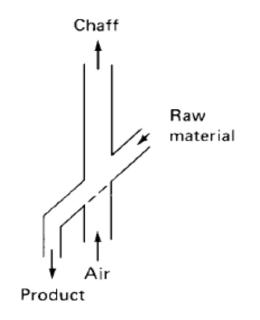
Fig. 1.1.2 Separation of chaff from grain by aspiration cleaning
