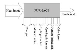
Ideally, all heat added to the furnaces should be used to heat the load or stock. In practice, however, a lot of heat is lost in several ways as shown in the figure.
