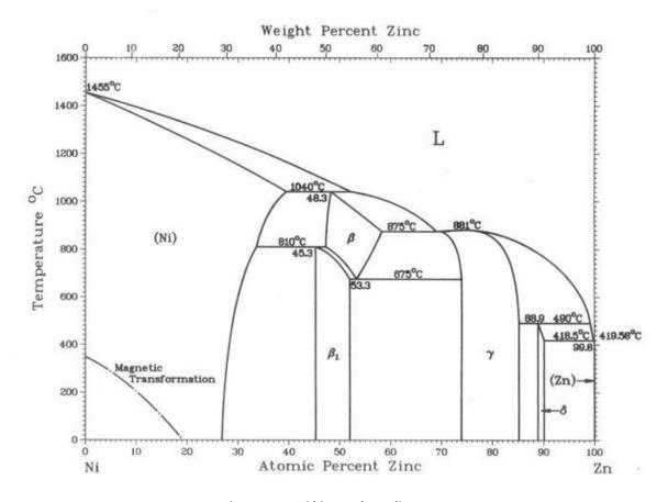
Fig. 1. Zn-Ni binary phase diagram
