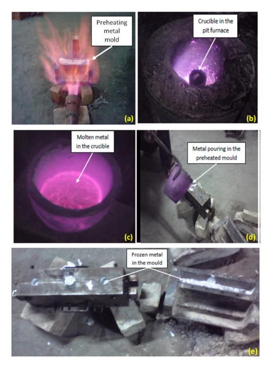
Fig. 2. Preparation of Zn-Ni Solder alloys (Casting Route)
