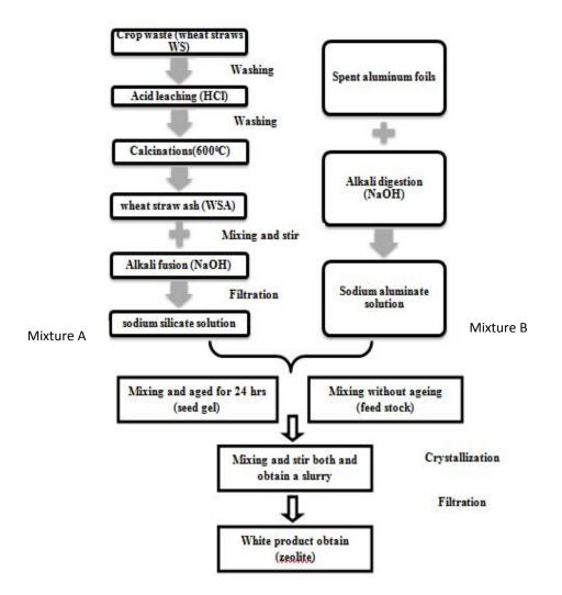
Figure.1. Flow diagram of zeolite synthesis
