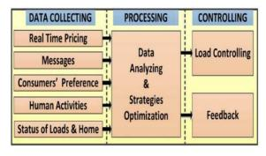
Fig. 4. Block diagram for dynamic price method
