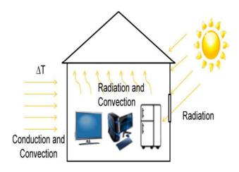
Fig. 2. HVAC heat load sources
