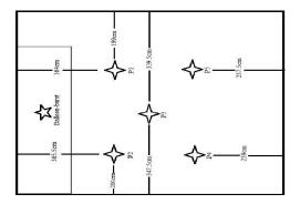
Figure 1 The Position of the Sound Source and the Microphone inside the Classroom.
