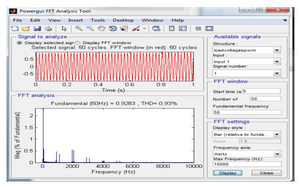
Fig.7 waveforms of showing the FFT analysis of load voltage of spwm
