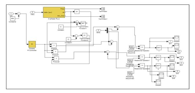
Fig 4 Simulink model of SPWM
