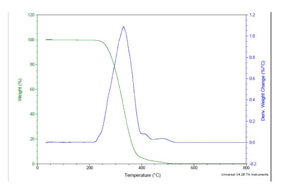
Fig. 12. TGA curve of 3L 10 wt% areca waste nylon fiber(areca:nylon=1:1) reinforced PP composites.
