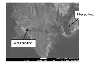
Fig. 15. SEM micrograph of tensile fracture surface of 3L 10 wt% areca waste nylon fiber (areca: nylon=1:1) fiber reinforced PP composite.
