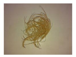
Fig. 1. Extracted Areca Nut Fiber
