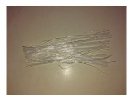
Fig. 2. Commercial Nylon Fiber
