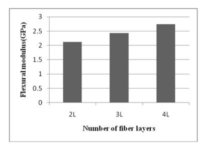
Fig. 10. Variation of Flexural Modulus with Number of Fiber Layers.
