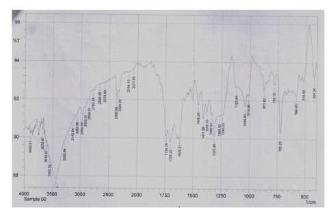
Fig. 4. FTIR Spectrum of Waste Nylon Fiber
