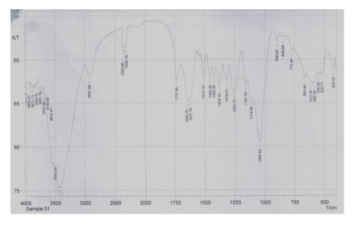
Fig. 3. FTIR Spectrum of Areca Nut Fiber
