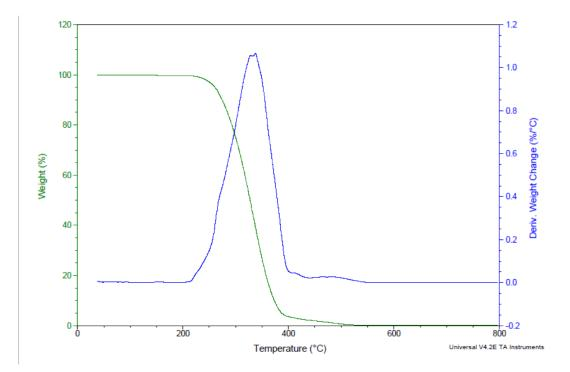
Fig. 13. TGA curve of 4L 10 wt% areca waste nylon fiber (areca:nylon=1:1) reinforced PP composites.
