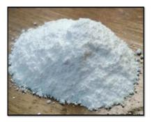
Fig. 7. Powder of cellulose acetate obtained
