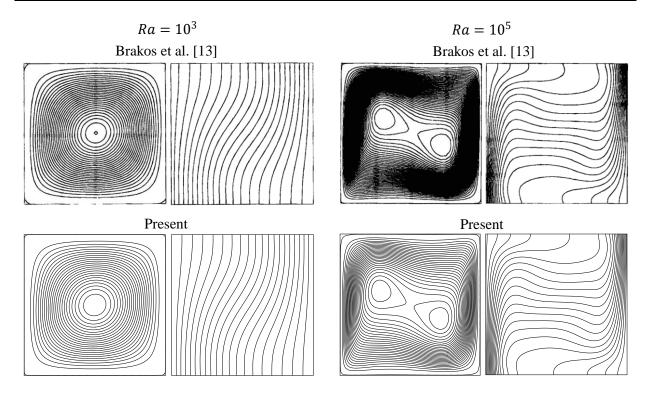
Fig. 2. Comparison of the streamlines and isotherms between the present results and that of Brakos et al. [13] at various Rayleigh numbers
