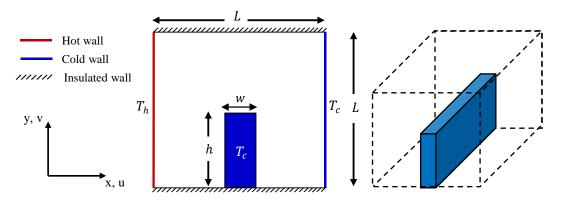
Fig. 1. Geometrical configuration and boundary conditions
