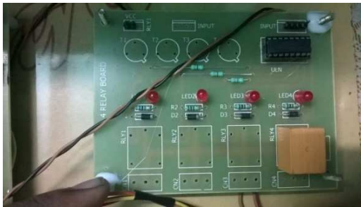
Fig .8 Relay circuit
