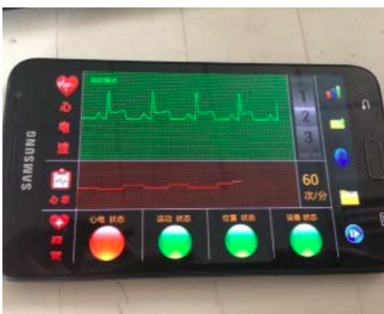
Fig 4.Output for ECG (P-Q-R-S-T waveform)
