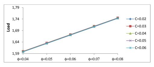
Figure- 4 Variation of Load carrying capacity with respect to  $\phi$  andC
