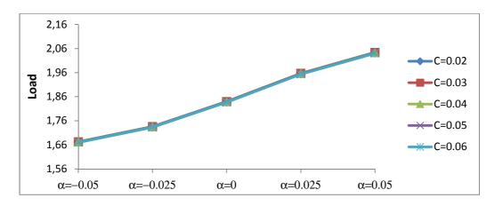
Figure- 10 Variation of Load carrying capacity with respect to  $\alpha$  and C
