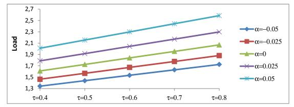
Figure- 14 Variation of Load carrying capacity with respect to  $\tau$  and $\alpha$
