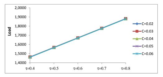
Figure- 5 Variation of Load carrying capacity with respect to  $\tau$  and C
