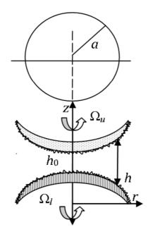
Fig. 1. The geometrical configuration of the bearing system
