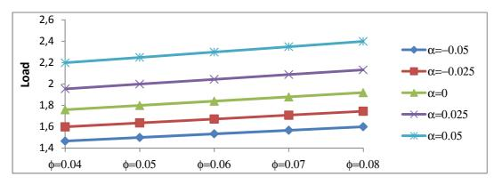
Figure- 13 Variation of Load carrying capacity with respect to  $\phi$  and  $\alpha$
