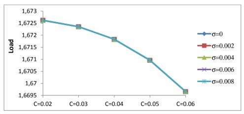
Figure- 11 Variation of Load carrying capacity with respect to C and  $\sigma$ .
