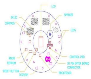
Figure2 Robot controller board
